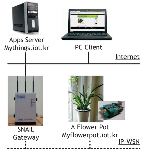
Figure 3: IP-WSN Testbed for the Demonstration
